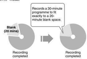
• The maximum recording time for JUST mode is equivalent to FR480 mode.
